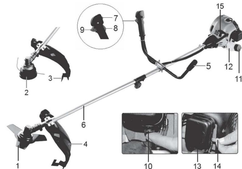
1. BLADE 3Z blade for grass, weed or brush cutting applications. Harness and plastic shield are required for blade operation
